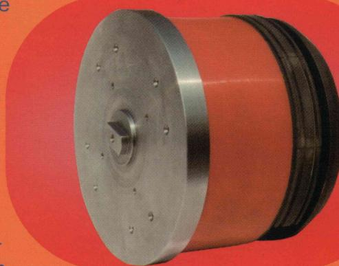
*The self centering expanding air RED-CHUCK is the only truly self-centering one and is particularly indicated for high speed jobs. When the air tube is inflated the axial expansion pushes out radially circular sectors that perfectly center the chuck into the core. The radial expansion of the air tube blocks the core that by adherence transmits the torque. Extremely light and easy to use.*
